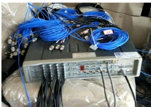
Fig 4 LMS data acquisition front end
